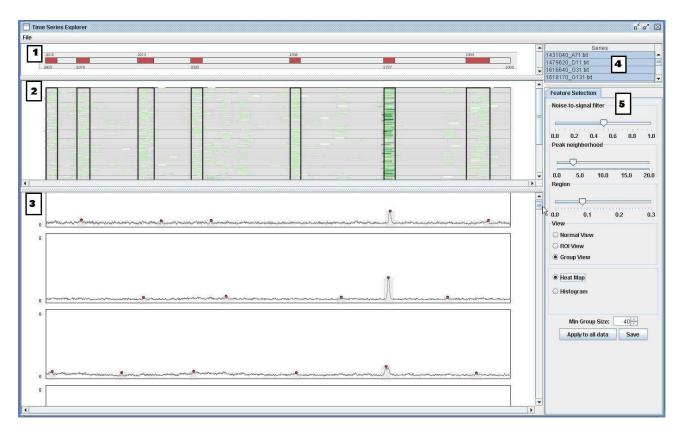
Figure 2: This shows the timeline panel (1), ROI panel (2), spectra panel (3), data panel (4), and the control panel (5) in grouped heat map view.
