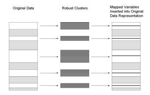
Figure 1. Mapping Robust Clusters to new variables to reduce dimensionality.
