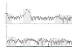
Figure 4: Peak identification. Dots mark identified peaks, gray boxes highlight the peak neighborhoods. Each plot represents one spectrum.
