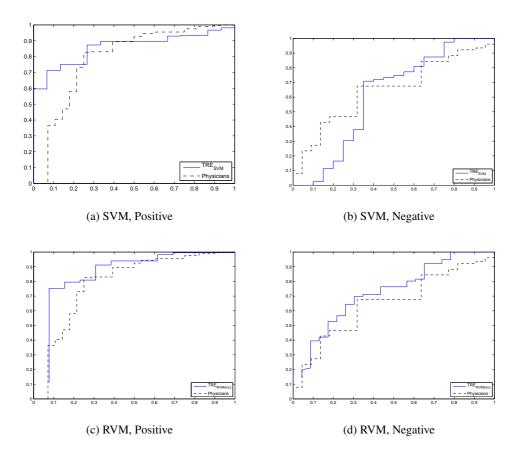
Figure 2: ROC curves for the transduction reliability measures for SVM and incremental RVM, using the CAD dataset and considering separately the positive and negative examples. For positive patients, each ROC curve depicts a ratio between reliable true positives on y-axis and reliable false positives (errors) on x-axis. For negative patients, each ROC curve depicts a ratio between reliable true negatives on y-axis and reliable false negatives (errors) on x-axis.
