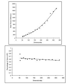
Figure 6. Scaling graphs of Difference in Fitness between CC and RCCC (top) and Percentage of Variables assigned to RCs (bottom) for increasing Dimensionality.
